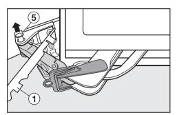
Push hinge pin (5) up and out from underneath.
